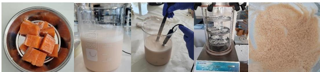
Figure 1. Production of trout protein isolate powder
